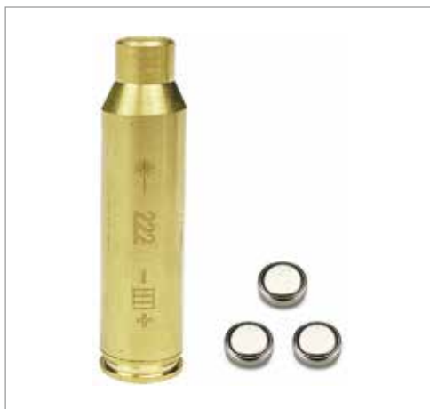
222 laser boresighter sighting length:39.5mm,bottom dia.9.5mm, top dia.6.3mm
